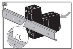
Ensure there is a good PE (ground) wire connection between the DIN rail and the BCM's PE contact.
