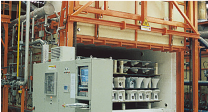
Intermittent shuttle kiln in the ceramics industry
