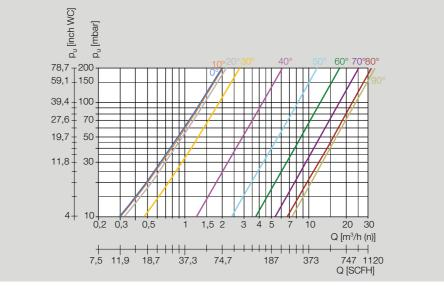
The characteristic flow rate curves have been measured with the valve closed.
