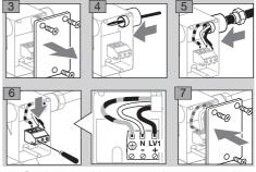
Set the solenoid actuator to the correct position ⊳ again and screw the hexagonal nut/cap tight if applicable.
